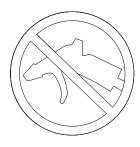
Drying and/or operating with compressed air destroys the flow sensor!
