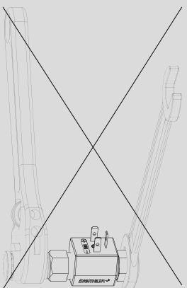
Important: Fittings should be mounted torsion-free, max. 10 Nm torque!
