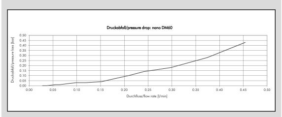
Test Settings: Medium: Water / Pressure: 2.0 bar
